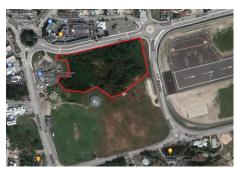
PHOTO SUBMITTED Cayman Air Traffic Visibility Requires Clearing of Land: Land near the cricket field will be cleared to remove the vegetation penetrating the flight path for landing and departing aircraft.
