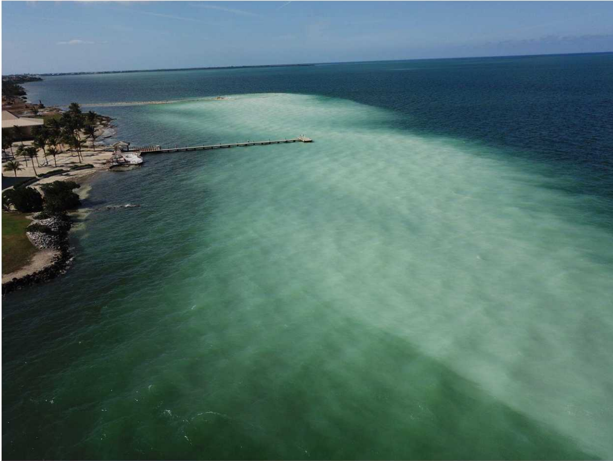
Figure 5: Drone imagery revealing the widespread impacts of dredging despite the installation of two layers of silt screens (Source: Submitted to DoE, 2018).
